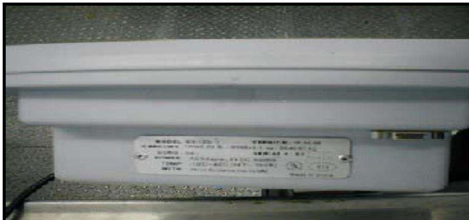
The New York NTEP Laboratory recommends that a scale with the identification located on an easily removed cover and electronic means of sealing still should have a physical security means to seal the cover to an integral part of the scale.
