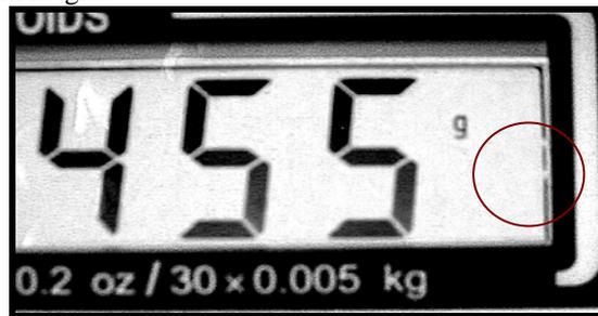
During their 2005 meeting, the Sector agreed that any proposal to specify the height of the weight display and units indications in NIST Handbook 44 should be limited to the Scales Code and should align with OIML R76 to the extent possible. The size requirements should be limited to weight indications visible to the customer in direct sale applications, the weight display should be no smaller than 9.5 mm, and the units display or marking should be no smaller than 2 mm.
