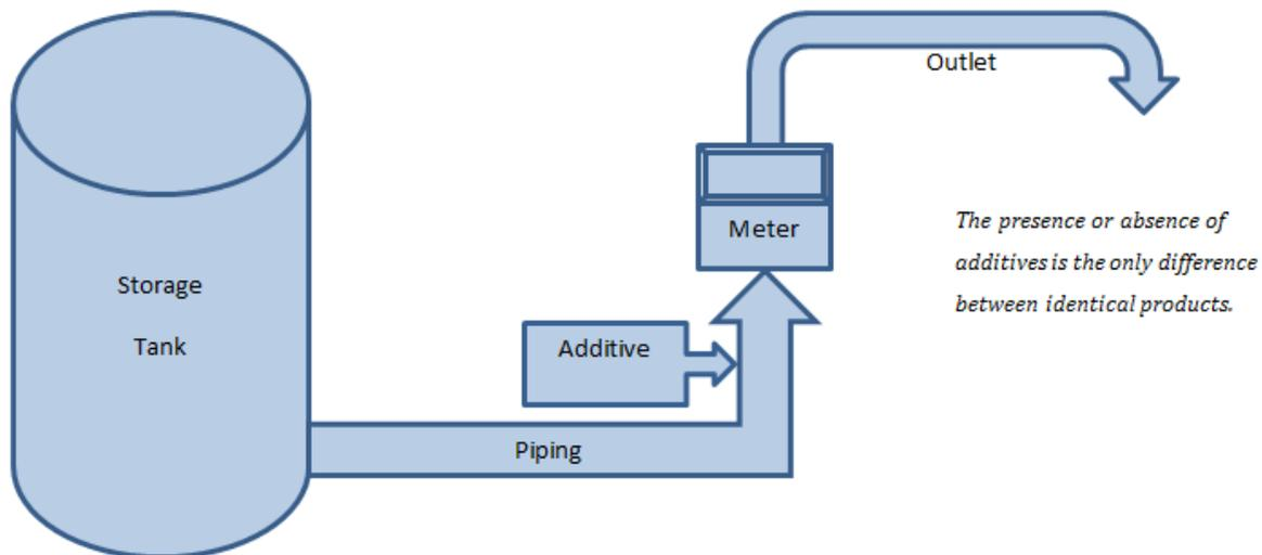
Identical products should be configured identically. Flow rates, and linearization factors at each flow rate, should be identical. Initially, only one product in a group of identical products needs to be physically tested, but it should be tested at all flow rates for which the meter is configured. On subsequent verifications, some of the flow rates may be verified empirically at the discretion of the regulatory official.
