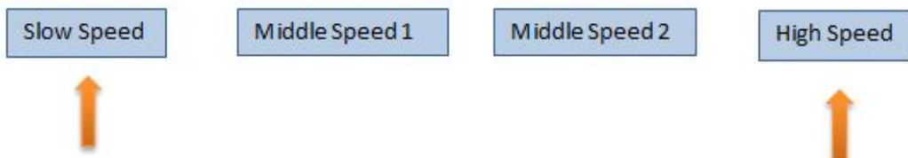
*Test the slow speed first, and then the high speed. The factors for the middle speeds should be between the high and low speed factors. The factors should be roughly linear.*
