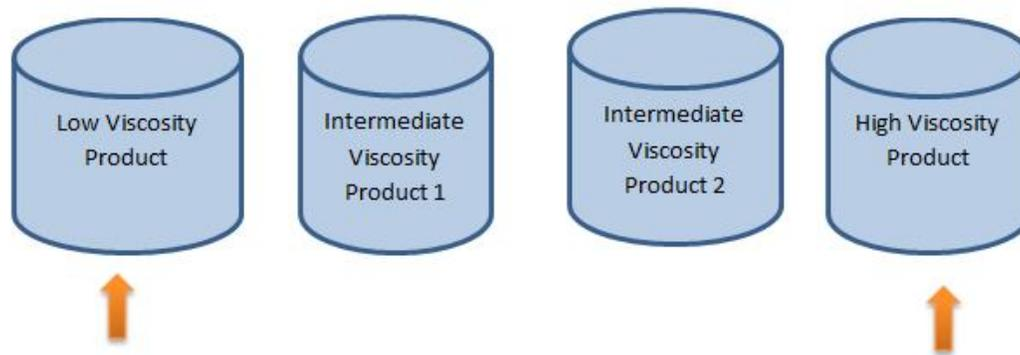
*Test the highest and lowest viscosity products, and then evaluate the linearization factors of the intermediate products. All products should have the same linearization factors at every configured speed, or the intermediate products should have factors which fall between the factors of the high and low viscosity products.*
