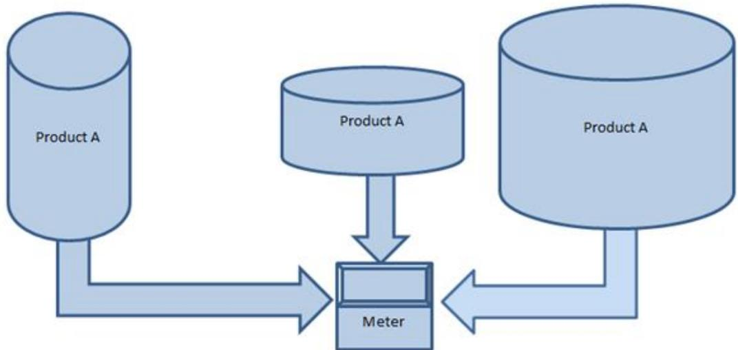
*The size and shape of storage tanks, the strength of different pumps, and the length and configuration of the plumbing, can affect the performance of some meters. Initial testing is needed to determine if the same product coming from different tanks can be considered to be similar, or if the product in each tank must be treated as if it was discreet.*
