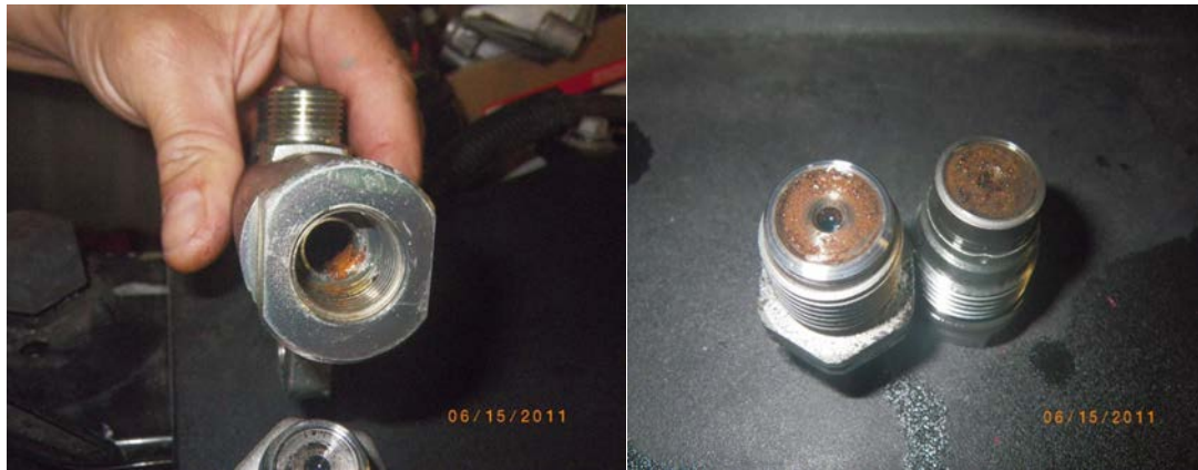
Figure 10: Common rail fuel system corrosion (photos courtesy of anonymous OEM)
