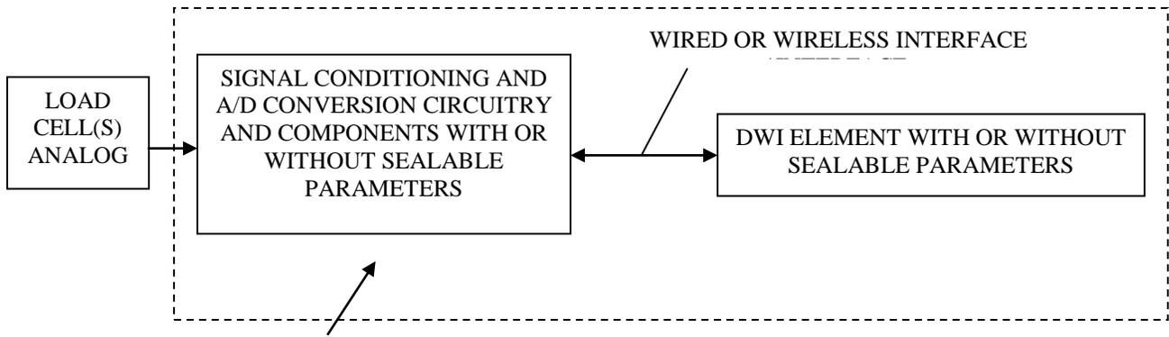
If NTEP Certification is for the signal conditioning element and the DWI element (the whole weight indicating element), use the Digital Electronic Scales (DES) examination procedure.
