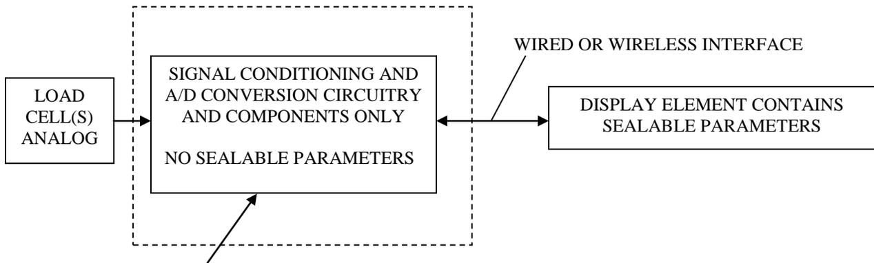
These checklists and test procedures apply if NTEP Certification is ONLY for this portion of the instrument.
