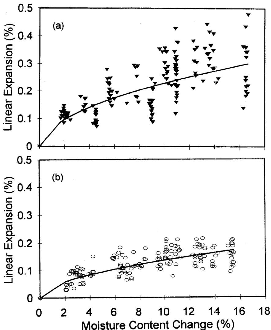
Figure 2. — Linear expansion as a function of change in moisture content from the combined data for all OSBs used in the study. (a) = perpendicular direction; (b) = parallel direction. The lines represent the fit of data. The average initial moisture content for all OSBs was 6.1 percent.
