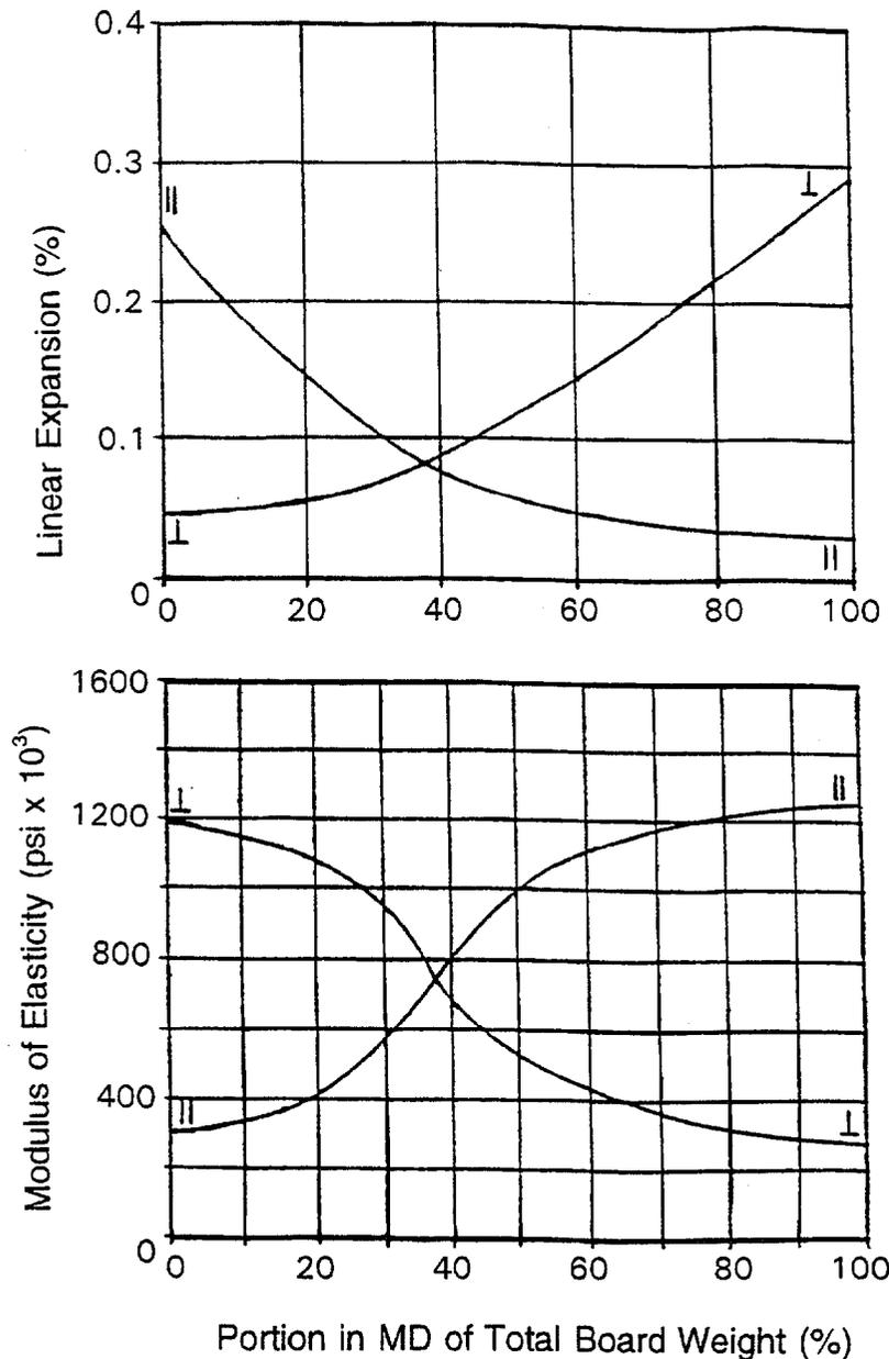
Figure 3. — Linear expansion (top) and modulus of elasticity (bottom) as a function of layer weight ratio adapted from Siempelkamp Corp. promotion literature. Linear expansion was measured from 50 to 90 percent RH at 20°C. || (parallel) and ⊥ (perpendicular) are with respect to the machine direction (MD). (1 psi = 6894 Pa.)
