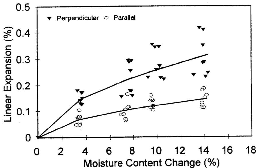
Figure 1. — A typical plot showing linear expansion as a function of change in moisture content. Data shown are for SPS with lines representing a power-law form fit. The average initial moisture content was 7.4 percent.
