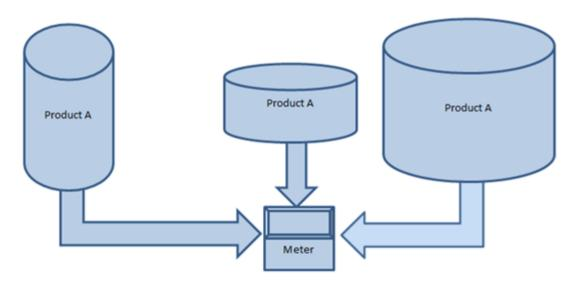
The size and shape of storage tanks, the horse power of different pumps, and the length and configuration of the plumbing, can affect the performance of some meters. Initial testing is needed to determine if the same product coming from different tanks can be considered to be similar, or if the product in each tank must be treated as if it was discreet.
