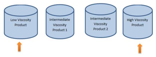
Test the highest and lowest viscosity products, and then evaluate the linearization factors of the intermediate products. All products should have the same linearization factors at every configured flow rate, or the intermediate products should have factors which fall between the factors of the high and low viscosity products.
