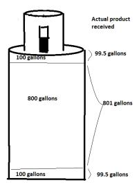
When calibrating at the normal and fallback speeds, the meter registers 200 gallons of product for the startup and shutdown, but actually delivers only 199 gallons. (99.5 gallons delivered for every 100 gallons registered at slow speed.) If the service technician calibrates the meter to zero at normal and fallback rates, the meter will actually deliver 801 gallons for every 800 gallons it registers at those rates.
